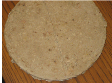
Figure 2. Cutting deficiency of ceiling tiles formulated with mattress cotton.
